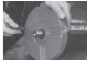
3 remove Non-Drive End oilseal levering with a screw driver
