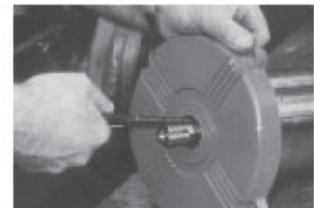
4 remove bearing retaining external circlip from the shaft
