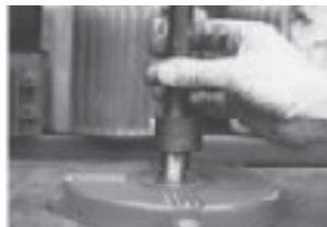
6 experience shows that the bearing housing and circlip will not be damaged. (This is an alternative method of endshield removal to picture 5)
