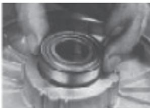
1 place endshield on flatsurface with inside facing upwards and insert the replacement bearing
