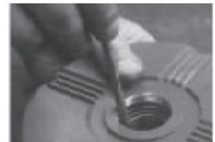
8 bearing can easily be removed using hand tools
